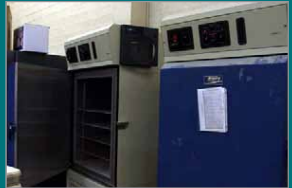
FIGURE 9 FREEZE THAW TESTING CHAMBER (NCMA PHOTO)
